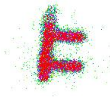
Fig. 9. Image reconstructed in real-time with Hicam Gamma camera coupled to a \pi shaped collimator and iodine source.
