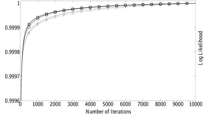
Fig. 5. Log-likelihood curves as a function of number of iterations. The different curves represent the log-likelihood for different scanning patterns of a pD-SPECT system. The scanning pattern is defined by its time ratio  $S$  which varies ranging from  $S = 0.45$ , to  $S = 0.9$  (from dark gray  $\square$  to light gray  $*$ ). All the curves are scaled with respect to their maximum value.
