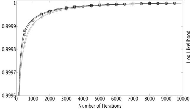
Fig. 4. Log-likelihood curves as a function of number of iterations. The different curves represent the log-likelihood for different levels of truncation. Truncation is caused by a limited detector size. The FOV diameter varies from  $w = 96$  to  $w = 36$  (from dark gray  $\square$  to light gray  $*$ ). All the curves are scaled with respect to their maximum value.
