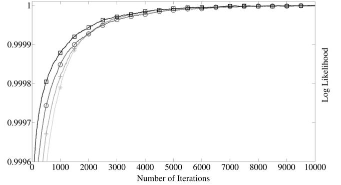
Fig. 3. Log-likelihood curves as a function of number of iterations. The different curves represent the log-likelihood for different collimator apertures:  $FWHM = 5.9 \text{ mm}$  to  $FWHM = 11.08 \text{ mm}$  (from dark gray  $\square$  to light gray  $*$ ). All the curves are scaled with respect to their maximum value.
