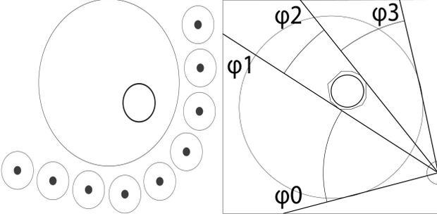
Fig. 6. A (left) position of pD-SPECT detectors - B (right) angular movement of a single pD-SPECT detector. Angular span of the FOV:  $\varphi_0 - \varphi_3$ . Angular span of the ROI:  $\varphi_1 - \varphi_2$ .
